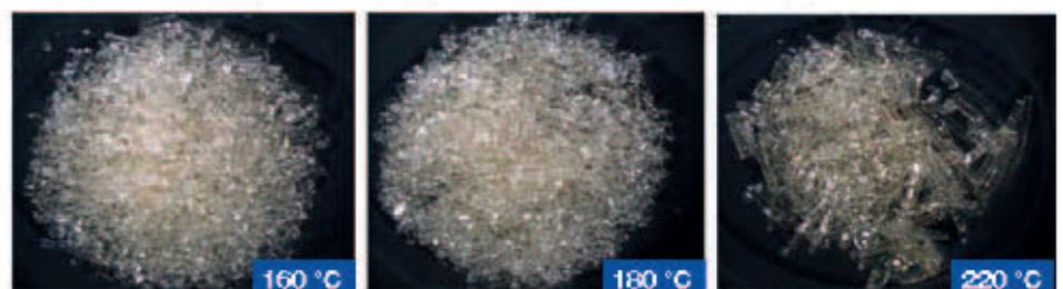
Kollidon® VA 64 extrudates obtained at different extrusion temperatures.
