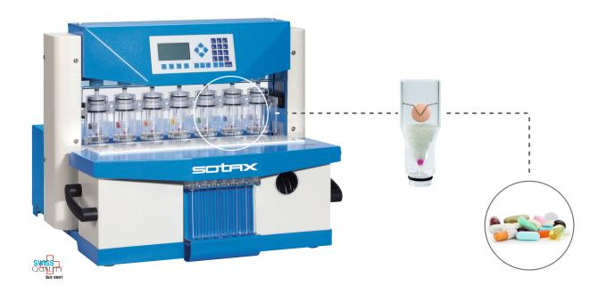
SOTAX CE7 Smart (USP4 Flow Through Cell) Allows you to see differences in your formulations that apparatus 1 and 2 simply do not show. Also widely recommended for poorly soluble, modified / extended release, and low dose products; Also been used for IVIVC studies and a growing range of dosage types
