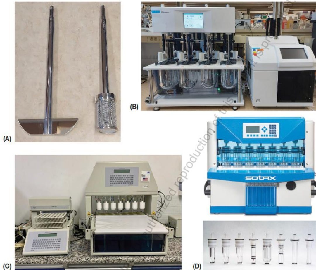
FIGURE 13-4 (A) USP dissolution apparatus 1 (Note the dye coming from the tablet in the basket); (B) USP dissolution apparatus 2; (C) USP dissolution apparatus 3; (D) USP dissolution apparatus 4.
